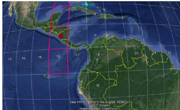
Fig.2 UTM Zones for Ecuador Source: Geo-ingeniería [11]
